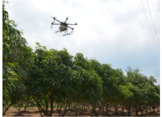
Demonstration of Spraying in mango orchard by using drone
